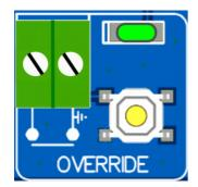
The TankStation has an override button and input. The input is activated when the two terminals are connected to each other. The button is physically wired across this input, so that pressing the button has exactly the same effect as connecting a wire across the two terminals.
