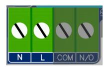
The PumpStation accepts an AC power supply in the range of 100VAC to 240VAC.
