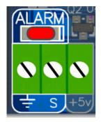
The device has an open-collector alarm output. This can be used to drive an input on a GSM Commander or provide local indication via a buzzer or LED.. When active, an internal transistor connects the "S" terminal to the " $\frac{1}{2}$ " terminal.
