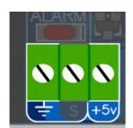
The PumpStation can be powered from a 5V DC voltage source, and shares a ground connection with the alarm output.
