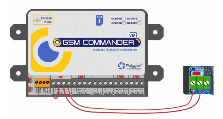
Bringing a GSM Commander into the mix creates a lot of interesting opportunities for monitoring the pump, but can of course also be connected to the alarm output on the PumpStation, allowing you to receive remote notifications of alarm conditions.
